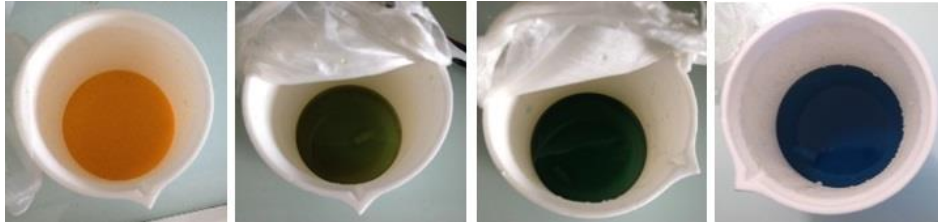
Figure 2.1. Evolution of the solution color (during the reduction of V 5+ (orange) in V 4+ (dark blue)).
