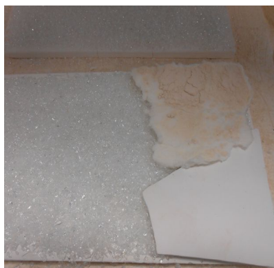
figure 7: Frit inside Kiln half Covered with Kiln Paper
