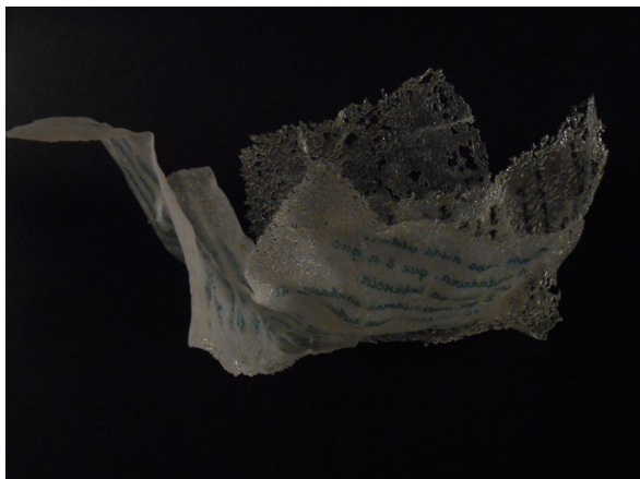
figure 21: Example 1 Result Slumping and Heat Gluing
