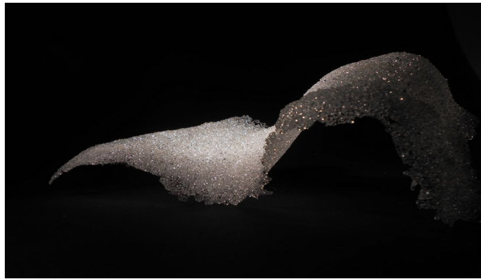
figure 16: Example Flat Piece Slumped at 725°C
