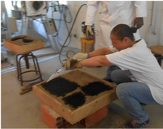
figure 32: Placing in Mould
