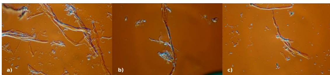
Figure 46. Observation of parchment fibres morphology from fol. 305, SC 4, by optical microscopy: a) several damaged fibres, at 160x magnification; b) partially flat fibre, at 300x magnification; c) ‘pearl on a string’ fibre with swollen and twisted areas, at 250x magnification.
