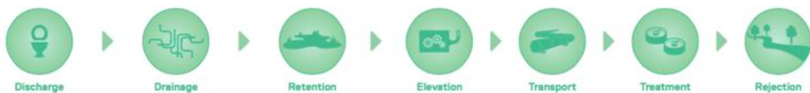
Wastewater Collection Process Flow
