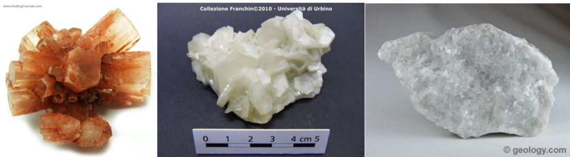
Figure 1 - Calcium carbonate crystals in nature, from left to right: Aragonite[9]; Vaterite[10]; Calcite[11]
