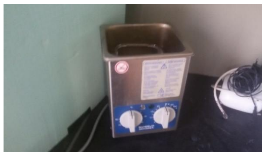
Figure 5 - Ultra-sonic machine, (Sonorex, Bandelin)
