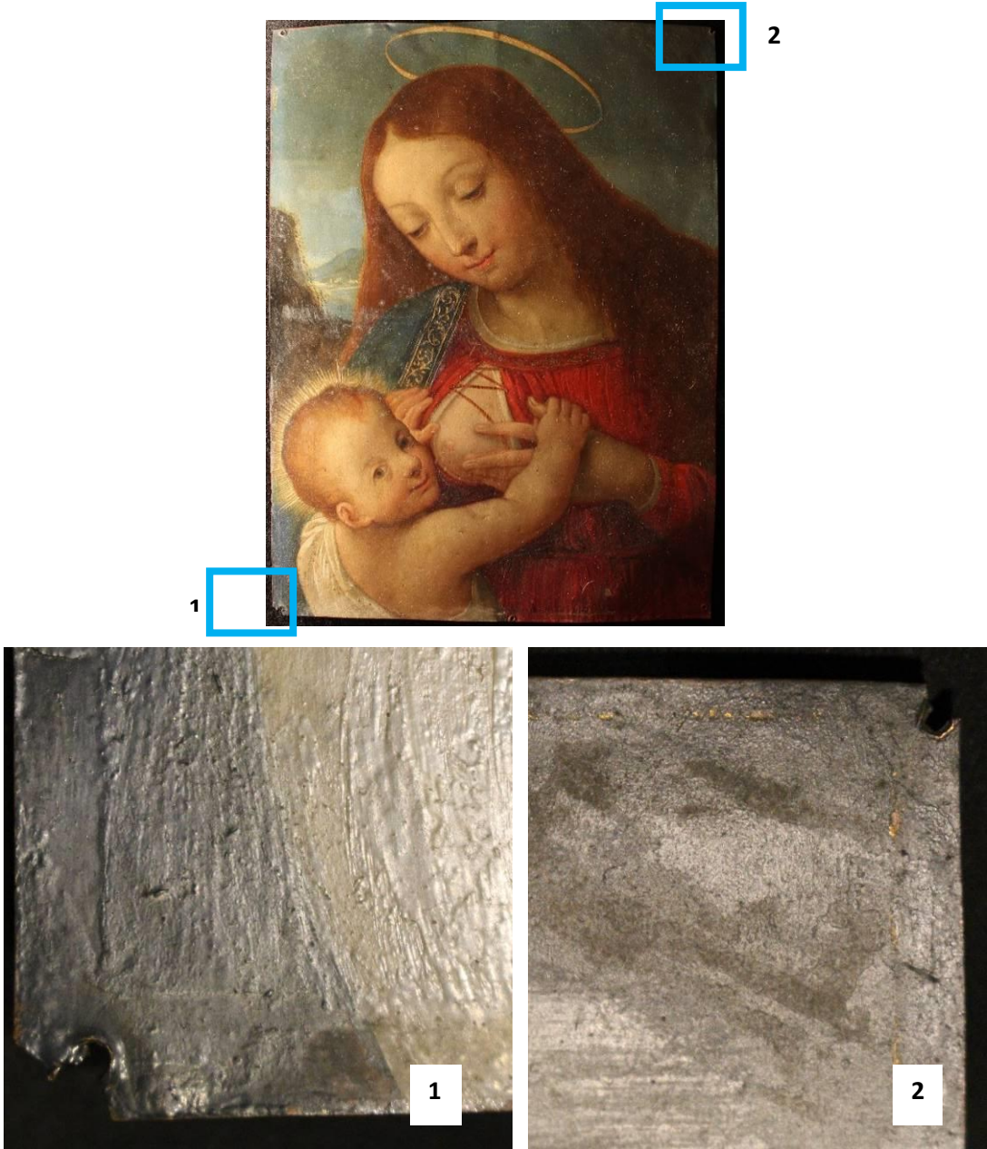
FIGURE V.1 – Sample of support losses in painting on copper PINT-K.
