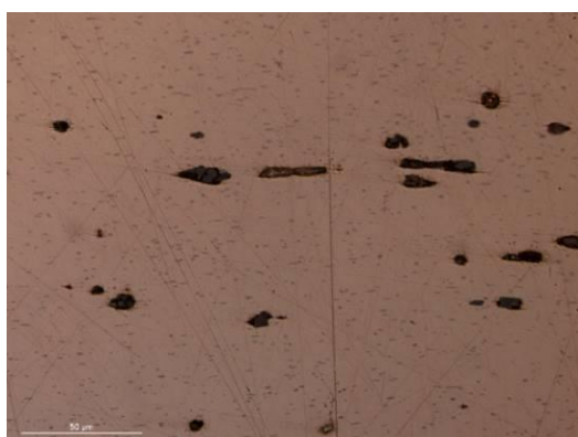
FIGURE 5 - PINT – K . Identification of cuprous oxide inclusions. Bright field illumination. Sample non etched.
