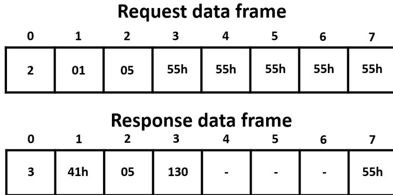
Figure 4.2: Request/Response CAN data frames.
