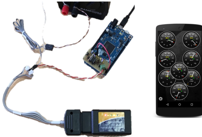
Figure 5.13: OBD Scanner Module to Arduino implementation.
