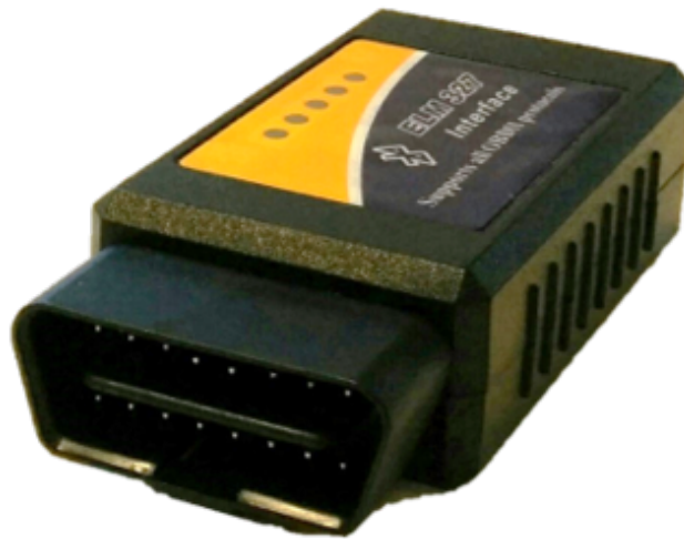
Figure 4.3: The ELM327 Interface Bluetooth version.
