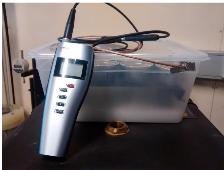
Figure 3.5- Samples placed in the plastic box for the sorption isotherms test
