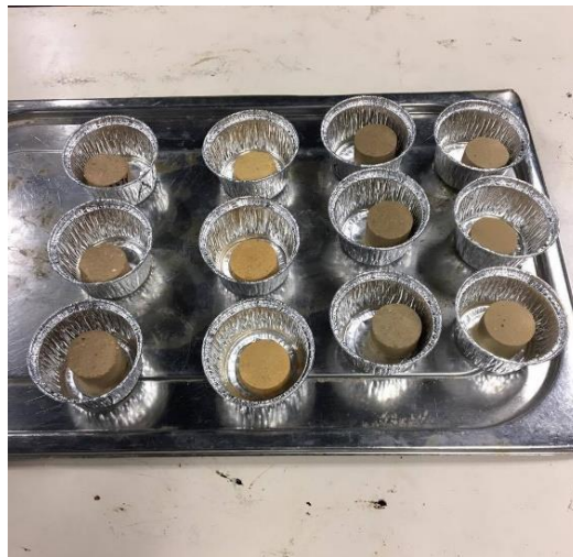
Figure 3.4- Example of samples used for the sorption isotherms test
