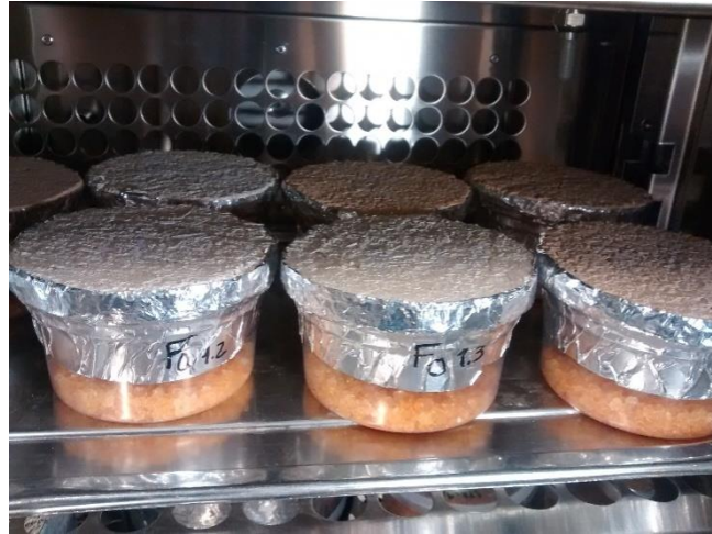
Figure 3.1- Dry cup samples with silica gel
