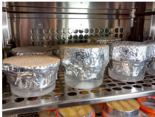
Figure 3.2- Dry cup sample with salt solution
