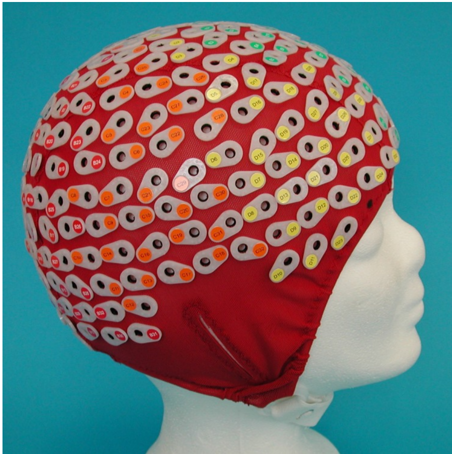
Figure 2.3: Electrode Cap with 256 electrode slots.
