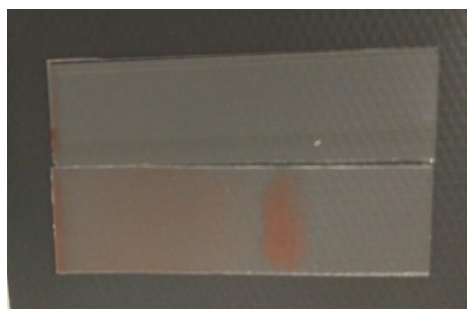
Figure 4.19 – Photograph showing the difference between Meyer rod (top glass) and newly designed method (bottom glass).
