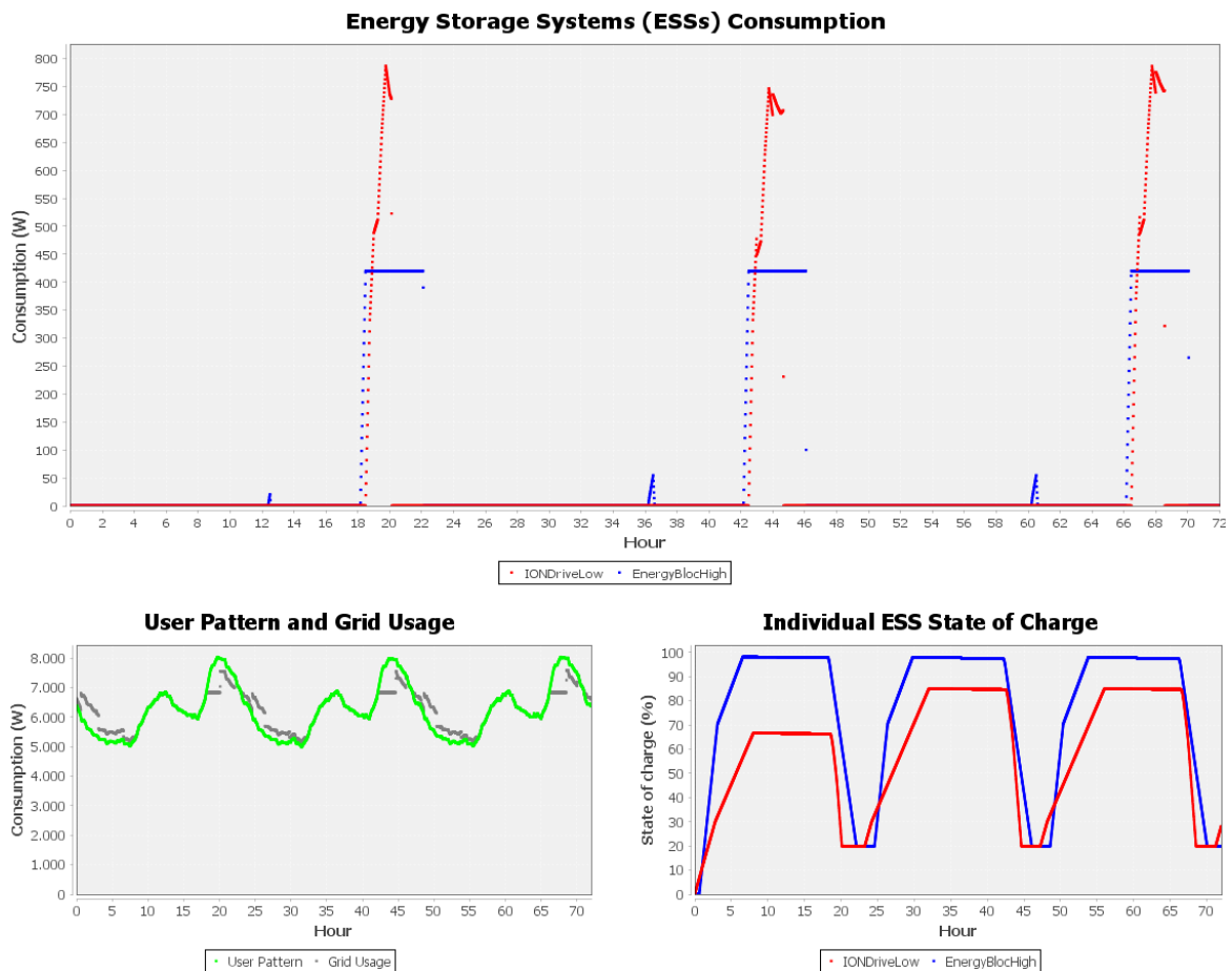
Figure 6.13 – Graphical results of a peak shaving simulation with three prices per day, two ESSs and a contracted power of 20.7kVA. This relates to a building with fifteen houses during the winter, simulated throughout three days.
