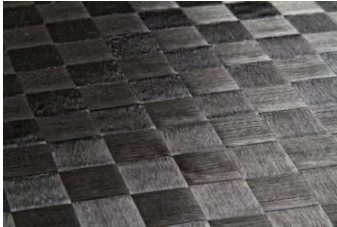
Figure 2.3 - Sample of a spread-tow carbon fabric [11]
