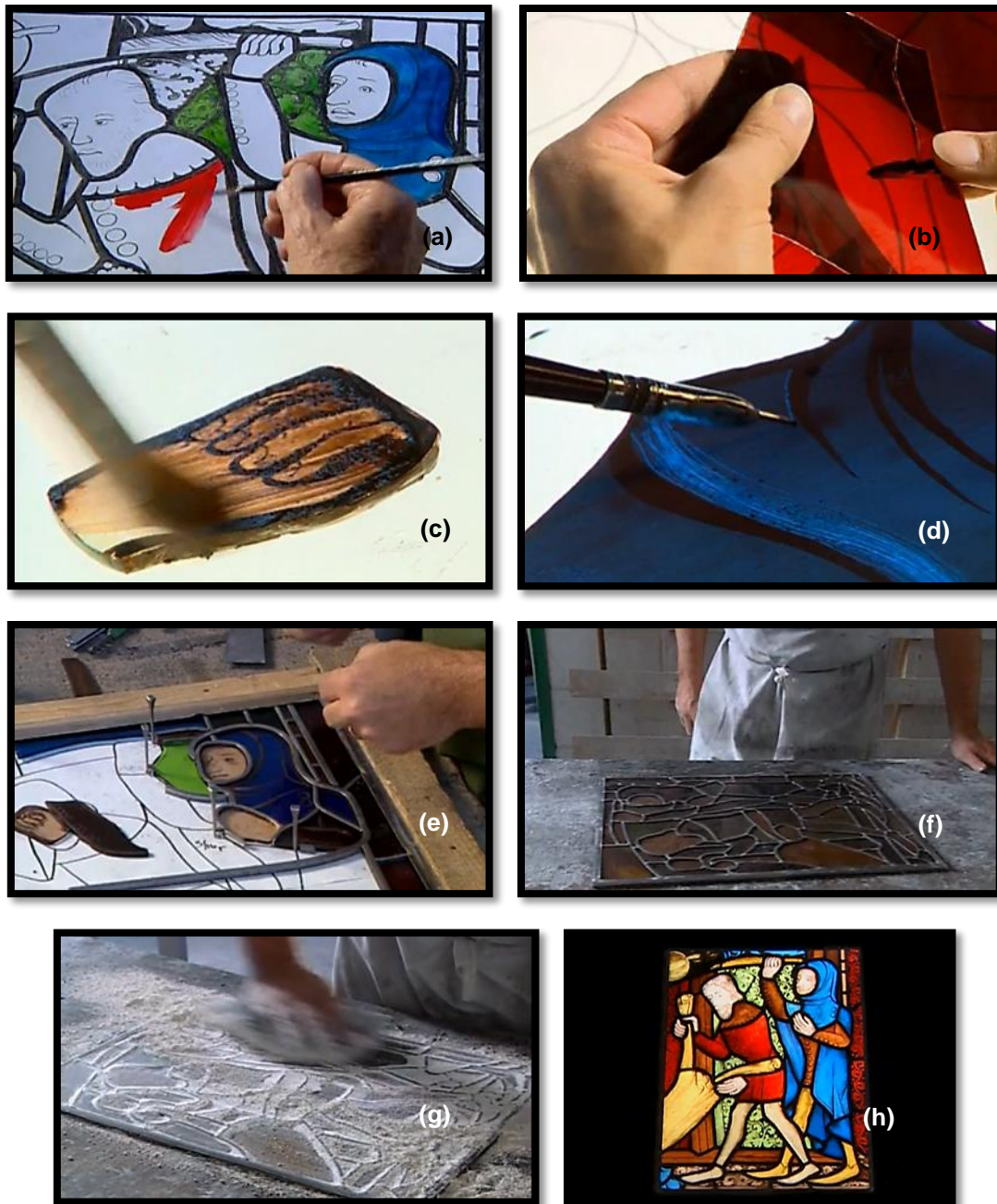
Figure 1.6: Methodology for making a stained glass panel. (a) In the first place, a full size cartoon is made, showing the lead lines around each glass fragment, as well as the colors and details to be painted on the glass; (b) then, the glass – colored or transparent – is cut to size, following the cut-lines from the cartoon; (c) also according to the cartoon, the grisaille painting is made, (d) using different tools and brushes, some of the details being made after the paint is dry. The fragments are fired in a kiln, for the paint – grisaille , yellow silver staining or, later on, enamels – to adhere to the glass surface. (e) By the time all the glass pieces are prepared, they are gathered on the cartoon, over a usually wooden base, and set together by lead came cut to size. (f) After completing this process, each junction is soldered, (g) and cemented on both sides in order to make the panel more resistant and waterproof, being left for a few days to harden. (h) Finally, the panel is complete. [Redol, 2003] These images are stills from the video “Making a stained glass panel”, that can be seen on the Victoria and Albert Museum website [ http://www.vam.ac.uk/content/videos/m/video-making-a-stained-glass-panel/ ], V&A©.
