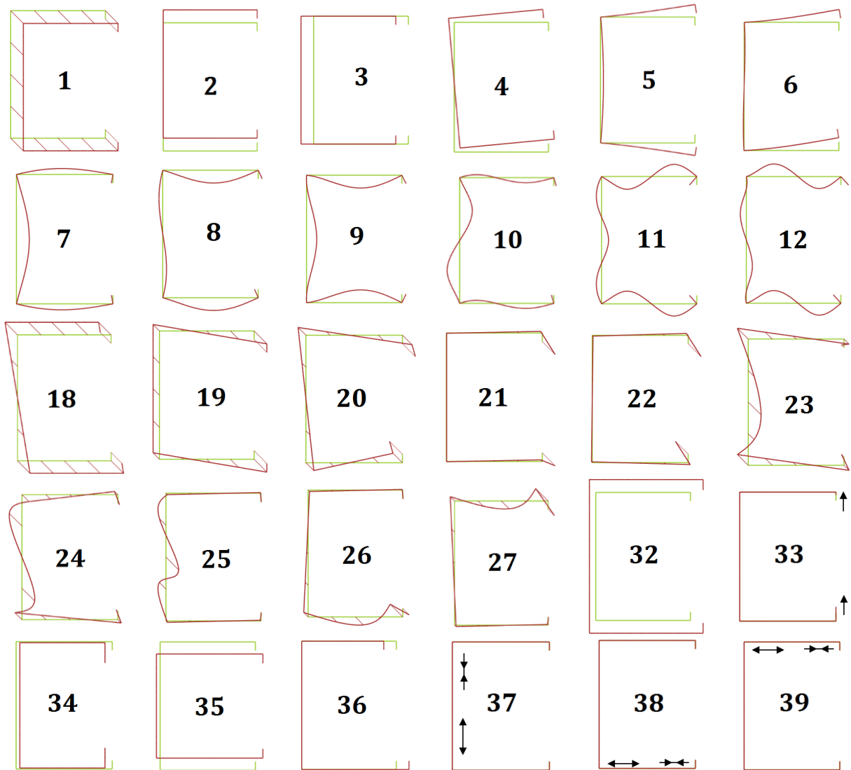
Figure 3: Lipped channel cross-section GBT deformation modes: (i) Vlasov modes (global (1-4), distortional (5-6) and local (7-17)), (ii) Shear modes (global (18-22) and local (23-31)) and (iii) Transverse Extension modes (isotropic (32) and deviatoric (33-36) global, and local (37-45)).
