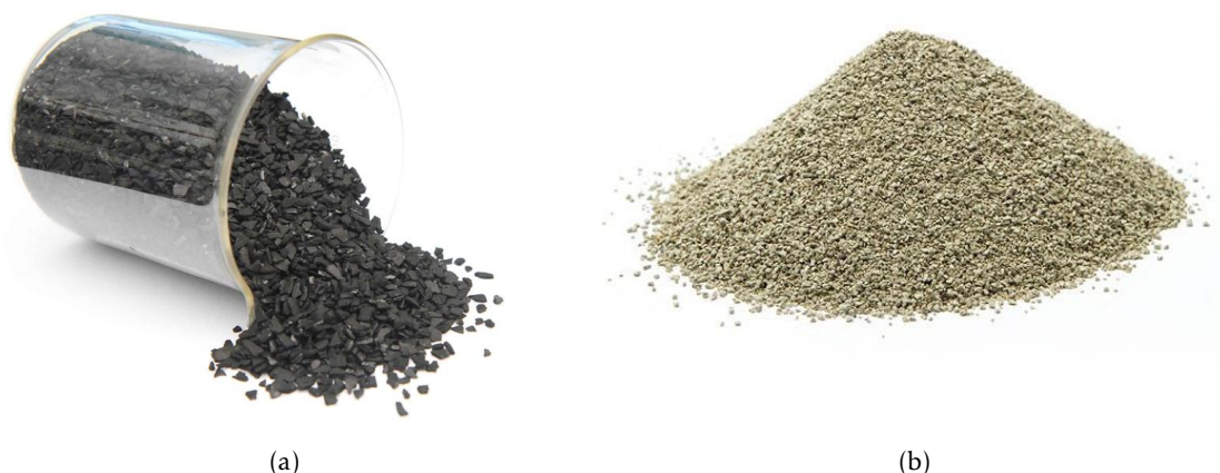
Figure 2.3: In (a), activated carbon [14]. In (b), zeolite [15]. These are the two most used and commercialized types of adsorbents.
