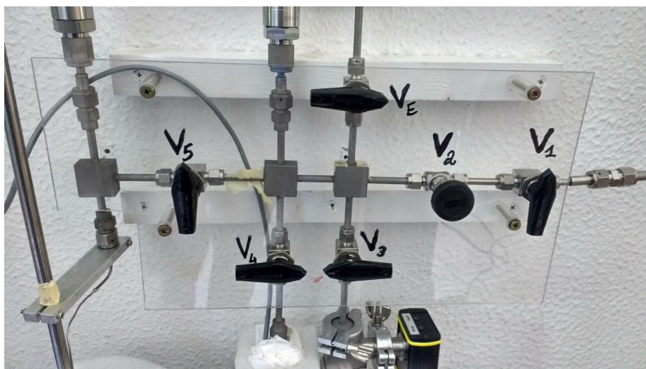
Figure 4.18: The manifold, fully wall mounted. Compare to figure 4.1 and note the support system described in subsection 4.2.2, figure 4.7, on the left after valve 5, as well as the insulation for the calibrated volume described in 4.2.3, after valve 4 in the bottom.
