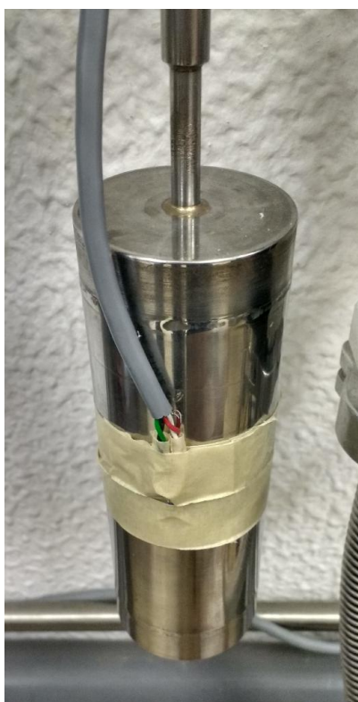
Figure 4.9: The calibrated volume, with the mounted thermometer C.
