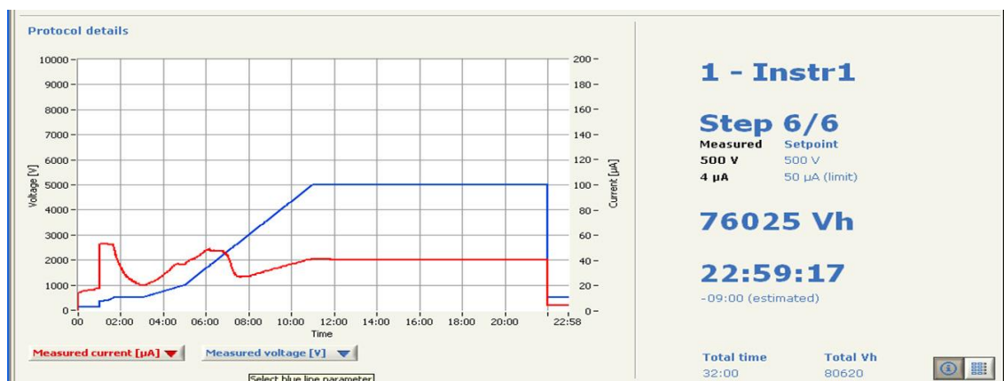
Figure 9. Isoelectric focusing run. Isoelectric focus was performed on a IPGPhor control software which records parameters such as voltage, current and volthours during the run.
