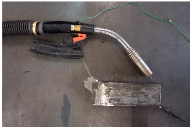
Figure 3.3 Connection of the voltage reducer circuit to the torch and substrate material
