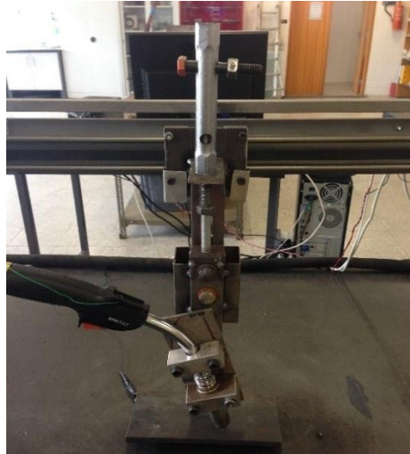
Figure 3.5 Torch clamping and height control
