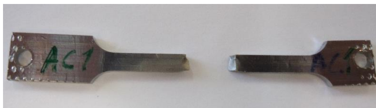
Figure 4.42 Specimen after uniaxial tensile test
