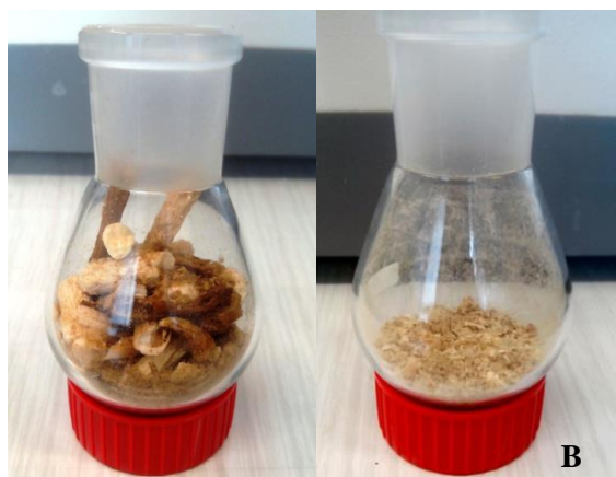
Figure 5.7: AP hydrolysates blend obtained from 11 different hydrolysis temperatures (A) and after homogenization (B).
