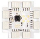
01 CORE MODULE Category: Board ATmega328 microcontroller
