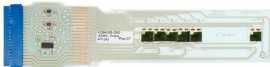
15 ISORG SLIDER Category: Component Six Organic Photodetectors.
