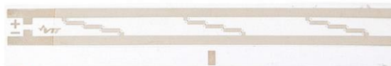
17 VTT LED STRIP Category: Component Red LED die chips on transparent PET: • 350 microns thick • Flexible
