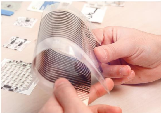
Thin and flexible polymer solar cell. You can cut it into the shape you want!
