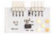
05 SENSOR MODULE Category: Board • Accelerometer – 3-axis analog output • Light Sensor (Phototransistor) • Temperature sensor (NTC)
