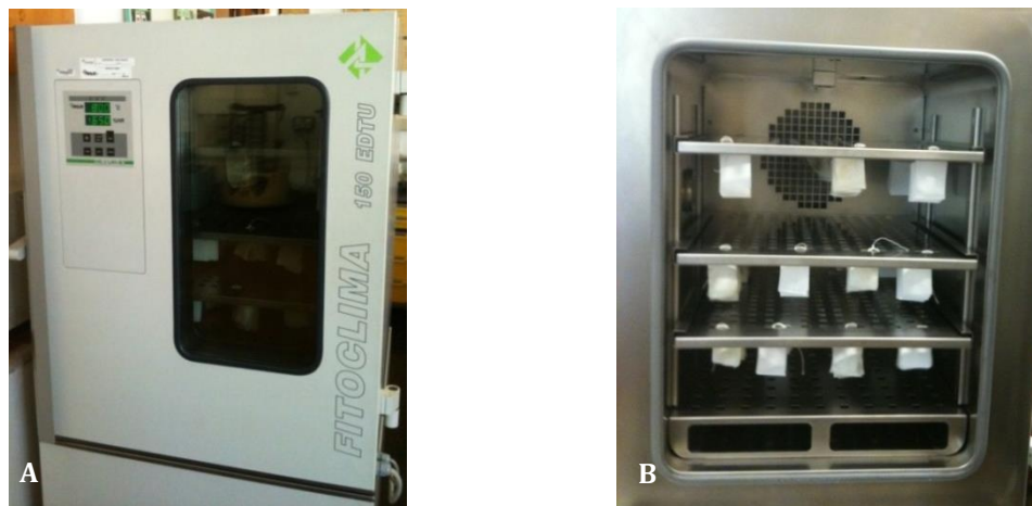
Figure 6.3: Climate chamber used for artificial ageing: closed (A) and open (B) with the suspended samples inside.
