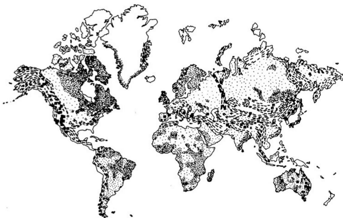
Figure 2.4 – Map showing the distribution of the large W and Sn skarn deposits and of the crustal elements; closed squares – W skarn deposits; crosses – Sn skarn deposits; dashed lines areas – Phanerozoic fold belts; dense dotted areas – Precambrian shields; lightly dotted areas – ancient platforms (Kwak, 1987).
