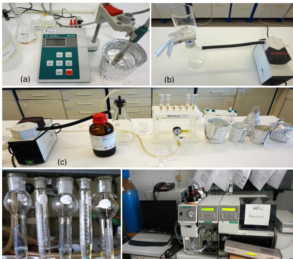
Figure 3.6 - Sequential analytical procedures for the aqueous samples: (a) pH adjustment; (b) Filtration; (c) SPE; (d) N 2 concentration; (e) HPLC analysis.
