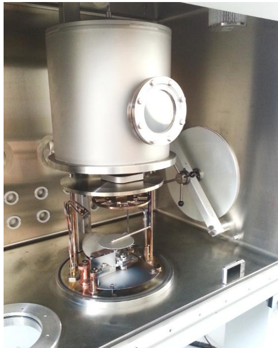
Figure A4: Picture of a Vactec thermal evaporation system. This system allows for the evaporation of a number of different metals, under a typical pressure of around 5 \times 10^{-7} mbar, supporting up to 9 samples at a time.
