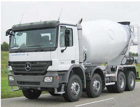
Figure 3.4.1.1 – Concrete mixer lorry (InvestConsult, 2015)
