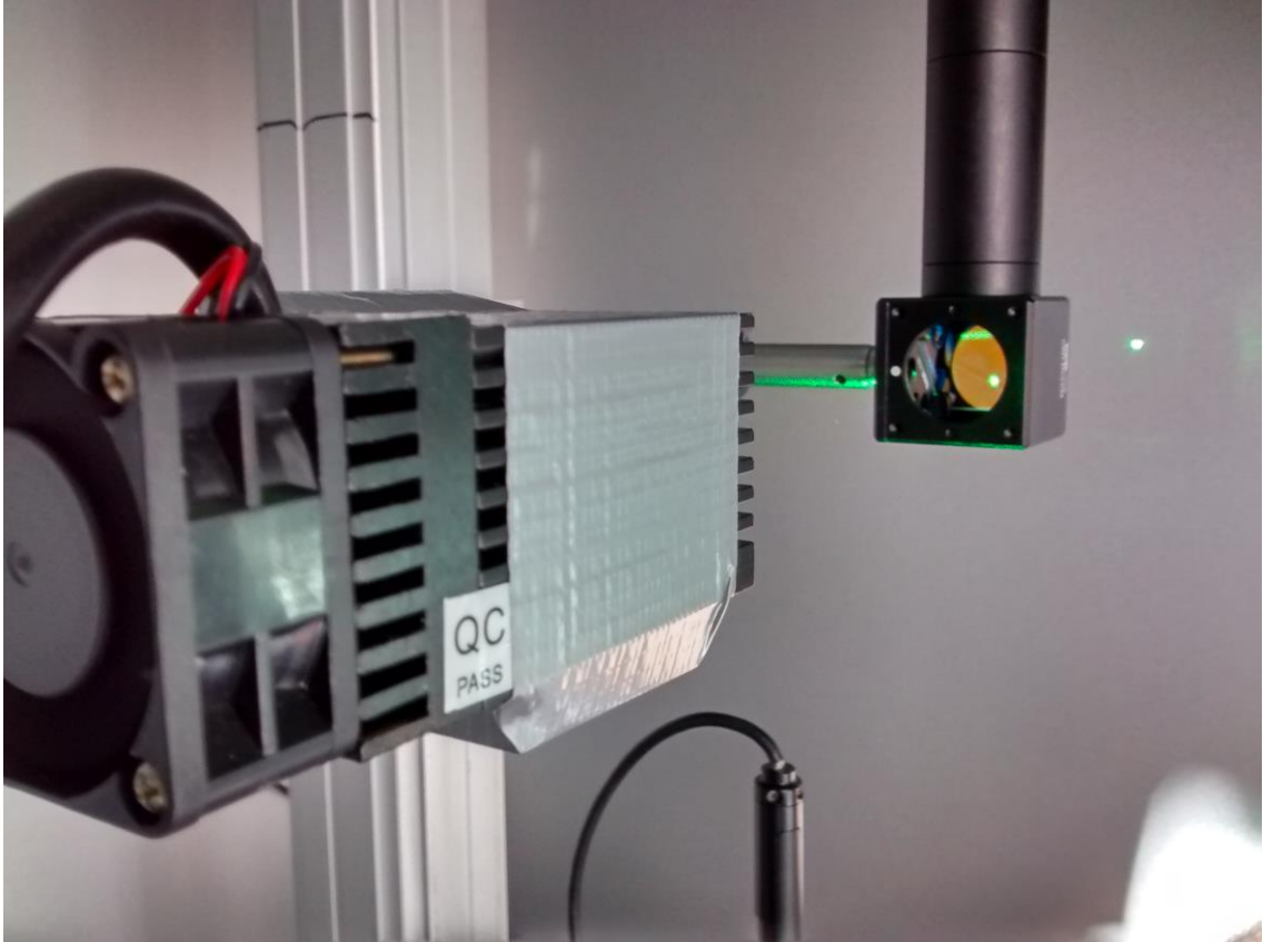
Figure 21 - Photograph of early structure depicting laser module aimed at the dichroic mirror after assembly.
