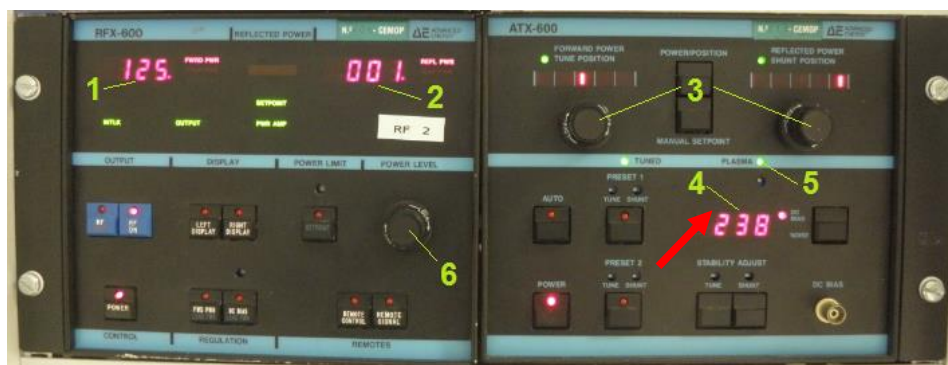
Figure 4.1 - RF magnetron control panel: (1) Forward power; (2) Reflected power; (3) Reflected power tuning; (4) DC bias display; (5) Plasma indicator; (6) Power wheel.
