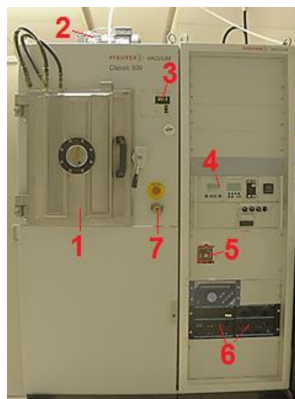
Figure 3.2 – RF magnetron sputtering system: (1) Vacuum chamber; (2) Rotation pump; (3) Pressure display; (4) Pump control panel; (5) Samples rotation control; (6) RF magnetron control panel; (7) Air admission valve.
