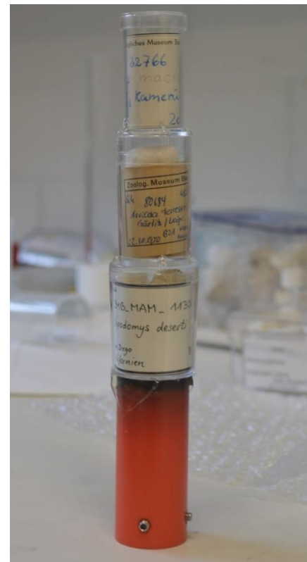
Figure 2.2 – Cylindrical plastic containers filled and glued, with specimens inside.
