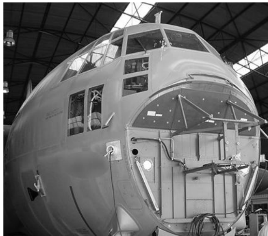
Fig. 5-2 - LOCKHEED MARTIN C-130 with the radome removed.
