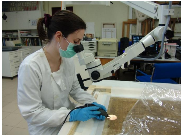
Figure V.17 – Trials with the Dremel® tool. The stereomicroscope was used throughout the removal of the lining adhesive.
