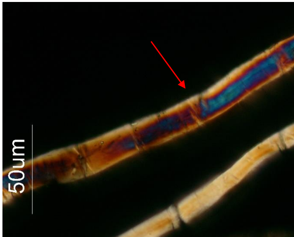
Figure IV.8 – Transversal view of the original canvas fibre under cross polarized light. The arrow indicates the cross marks.
