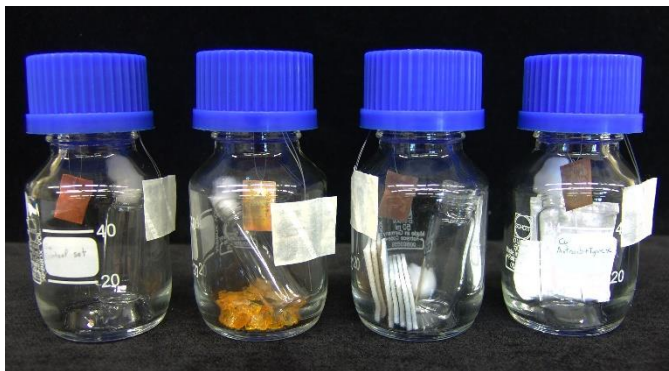
Figure VII.1 - Oddy test bottles of the copper coupons. From left to right: Control, Orange silica gel, Artsorb® and Tyvek® covered Artsorb®.
