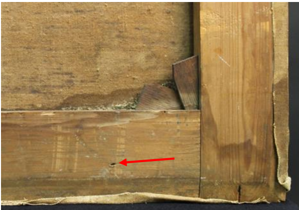
Figure II.3 –Water mark in the stretcher and canvas and mould growth on the canvas. The arrow indicates one of the insect exit holes present in the stretcher.
