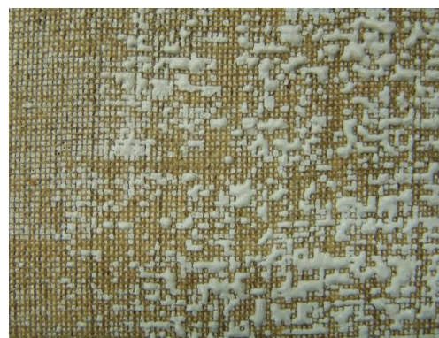
Figure 4 - Ground sticking out at the back of a canvas sample from HART Project. Ground was composed by lead white and barium sulfate in oil and the size used was fluid. Photography taken by the author.
