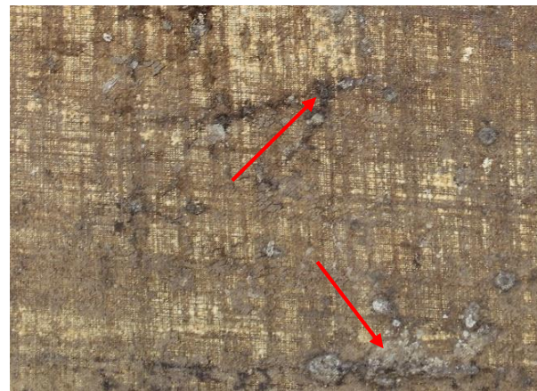
Figure VI.9 – Mould growth on the original canvas and in the lining adhesive. The arrows indicate two sampling areas.
