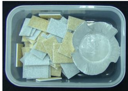
Figure VII.2 - Box for pre-conditioning the Artsorb® with the metal container to deliver water.
