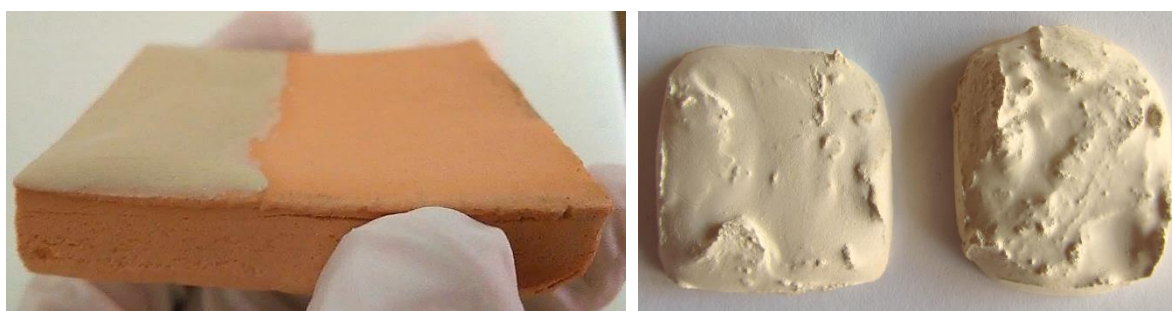
Figure 3. Types of samples prepared. Left: paste applied on a reference ceramic substrate “Mortágua” 5 x 5x 1 cm and right: pure paste monolith.
