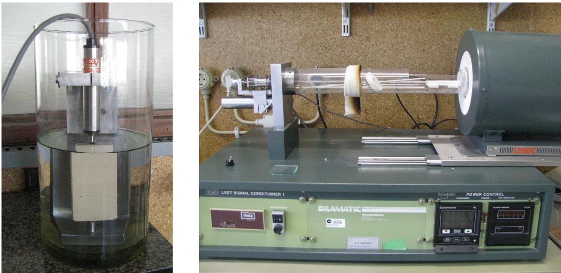
Figure IV. Physical and mechanical characterisation of geopolymer pastes. Left: hydric expansion test; right: thermal expansion test.
