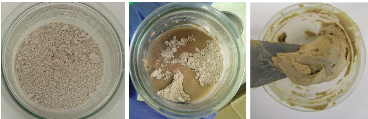
Figure I. Preparation of geopolymer paste. Left: metakaolin in powder; centre: addition of alkaline solution; right: final paste of geopolymer.
