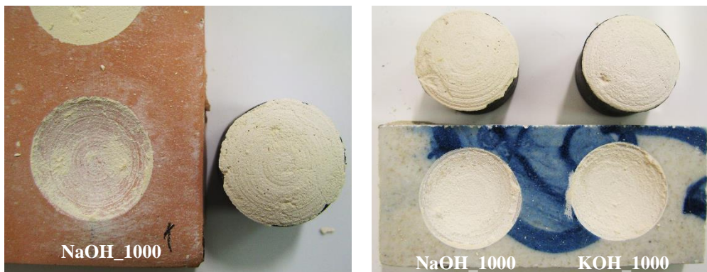
Figure 20. Adhesion strength test of geopolymer pastes. Left: paste applied on the reference ceramic substrate “25% CaO” and right: pastes applied on historical azulejos cured at 21 °C.
