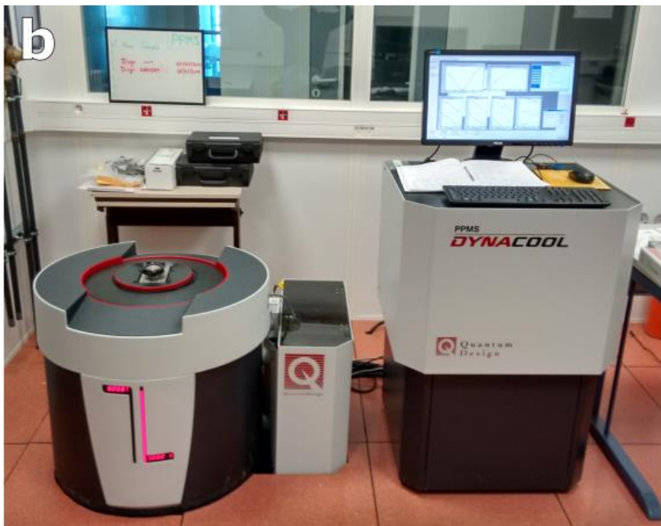
Annex Figure 7 - Quantum Design's PPMS Dynacool system. a) The puck used has three channels. Three samples can therefore be measured at the same time. b) The PPMS Dynacool allows programmed measurements at low temperatures (1.8K) and high magnetic fields (9T).
