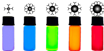
Figure 1.8: Relation between the size of the CQDs, with capping agents involving them, and the emitted color of the corresponding suspension, under irradiation.
