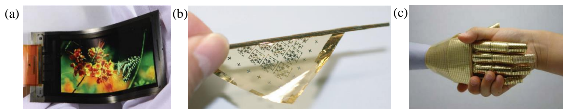
Figure 1.4 – Few promising organic electronics applications: (a) flexible active matrix organic light-emitting diode (AMOLED) [23]; (b) organic and flexible TFTs [24]; (c) Sensors based on organic material [25].
