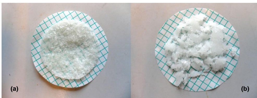
Figure 4.6: Appearance of the membranes after digestion: (a) anion exchange membrane, (b) cation exchange membrane
