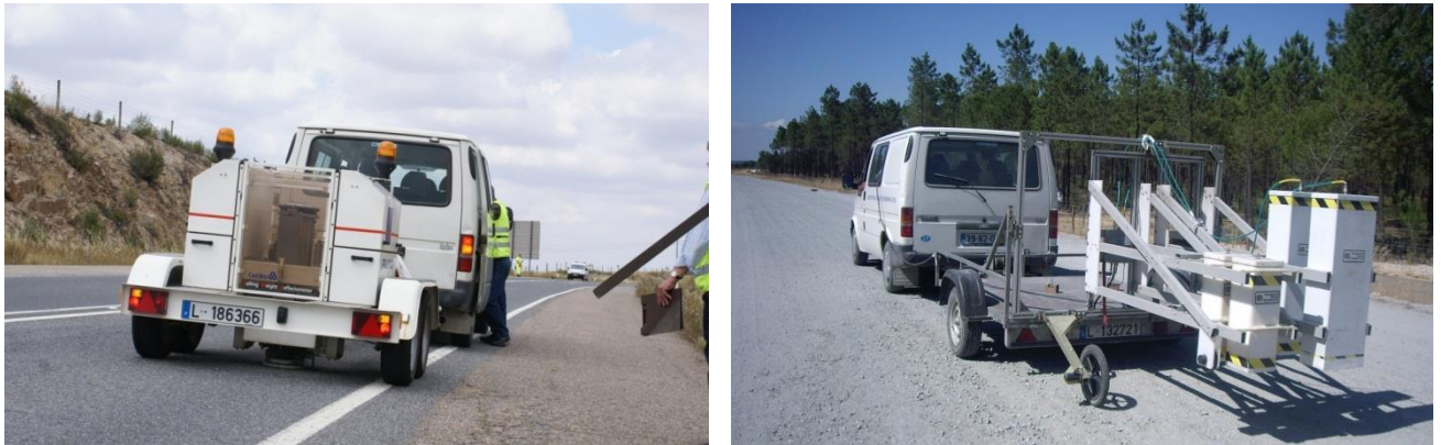
Figure 2.1 – LNEC’s FWD (on the left) and GPR (on the right) equipment
