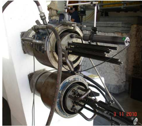
Figure 5.16: Detail of the VSL stressing jacks
