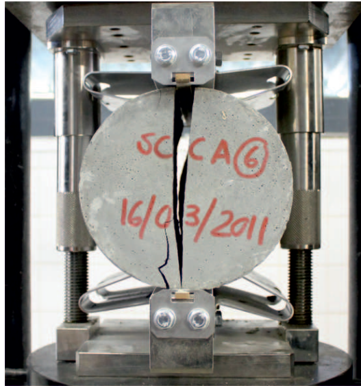
Figure 2.29: Failure mode of a HPC cylinder in the tensile splitting test
