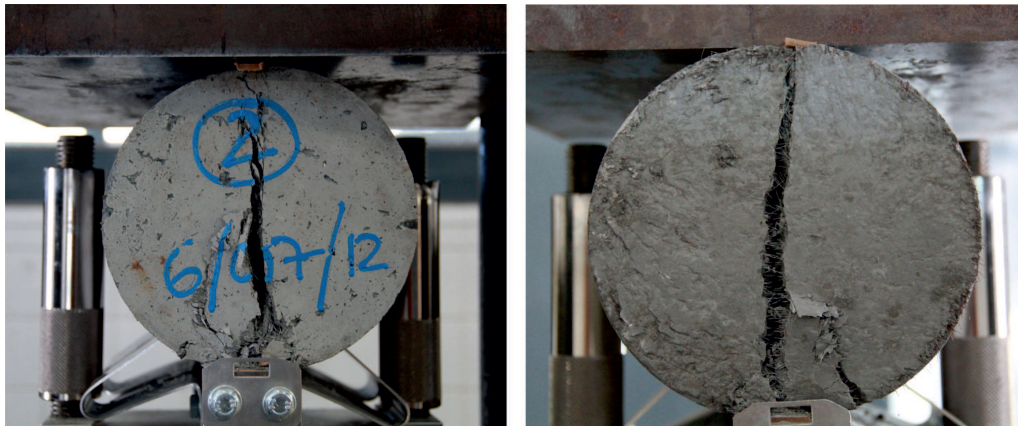
Figure 2.30: Failure mode of a HPFRC cylinder in the tensile splitting test
