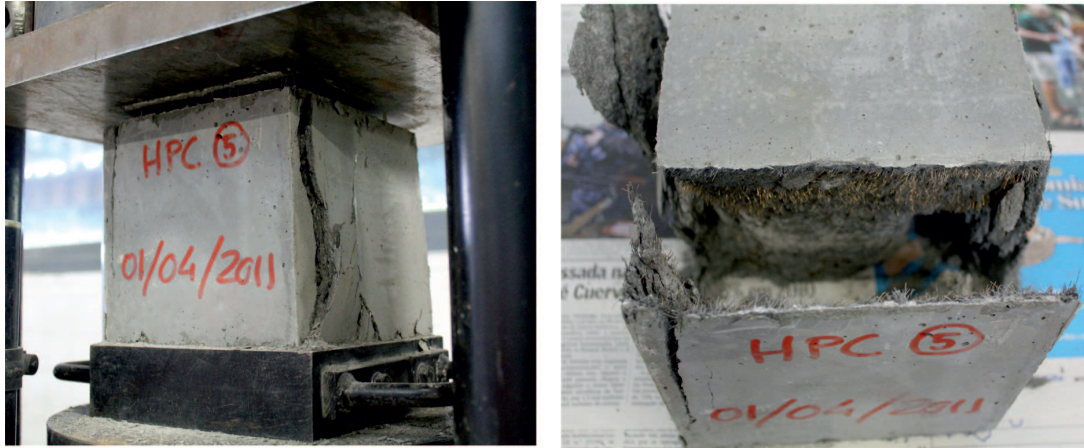
Figure 2.24: Failure mode of a HPFRC cubic specimen
