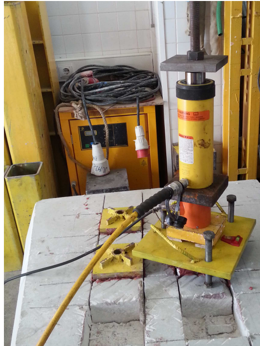
Figure 5.88: Pull-off test setup
