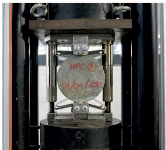
Figure 2.28: Test setup for tensile splitting tests
