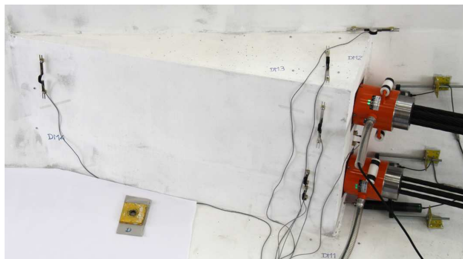
Figure 5.14: Detail of the monitoring equipment in the anchorage blister
