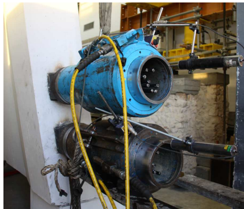
Figure 5.17: Detail of the STRONGHOLD stressing jacks
