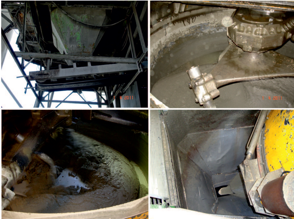
Figure 2.12: Production of HPFRC on site
