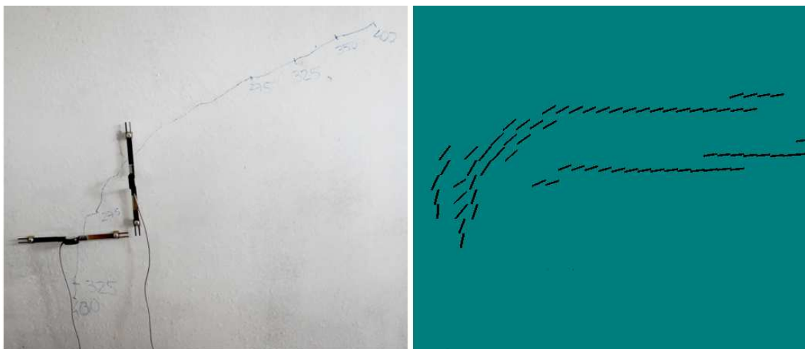
Figure 5.111: Comparison of cracking on the underside of the slab at the end of the experimental test
