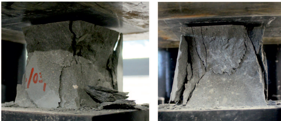
Figure 2.22: Failure mode of a HPC cubic specimen
