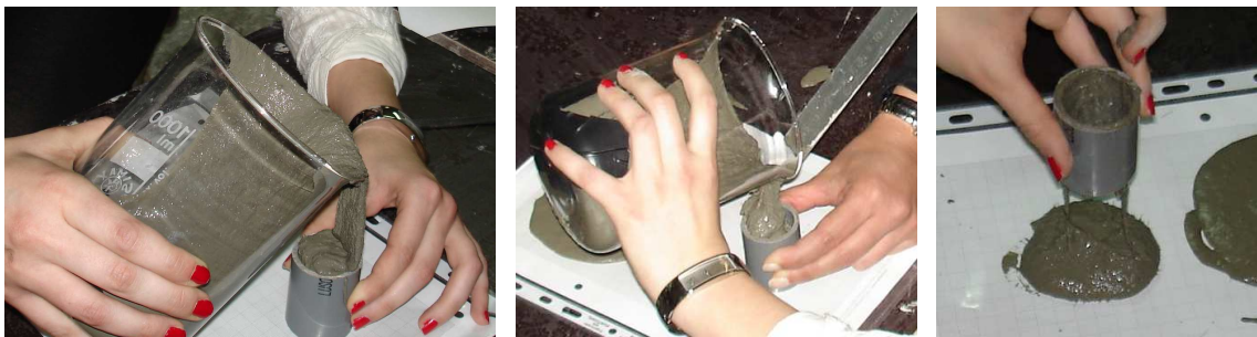
Figure 2.16: Performance of mini-slump test
