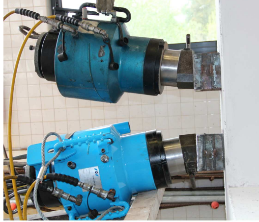
Figure 5.47: View of the VSL stressing jacks
