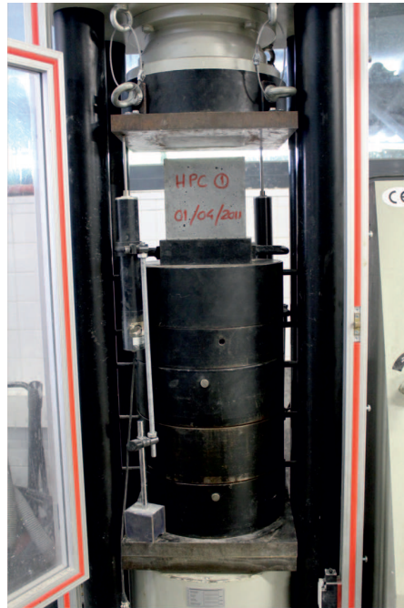
Figure 2.21: Test setup for uniaxial compression tests
