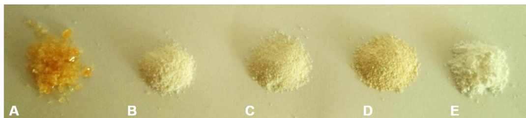
Figure 9. A- TiO 2 nanoparticles before calcination, and after a short sintering process (120°C, 1h and ramp: 60°C/h). B- Synthesized powder from calcination at 400°C. C- Synthesized powder from calcination at 520°C. D- Synthesized powder from calcination at 625°C. E- Commercial anatase (Degussa P25).
