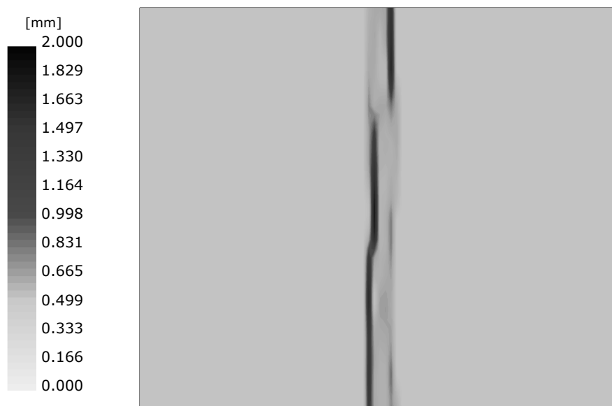
Figure 4.58: Cracking on the bottom surface of the numerical model B
