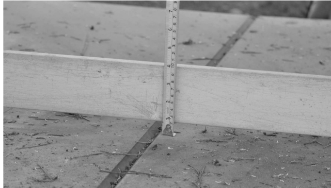
Figure 4.8: Residual deformation's measurement
