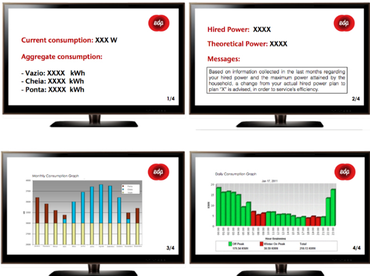
Figure 9 – Image representing an example of how EDP's provided feedback would be displayed in the television screen and seen by the consumer
