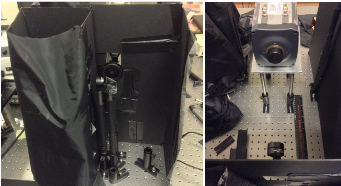
Figure A.2 Photographs of the system after the removal of the telescope, installation of the sensor and proper shielding. The light source (the tip of optical fibre) is completely shielded with black card and a soft plastic fabric.
