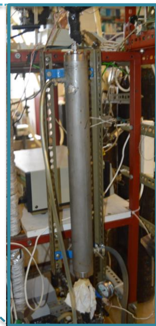
Figure 2.13 – Separator (oil/carotenoids extraction)/ Reactor (enzymatic transesterification).
