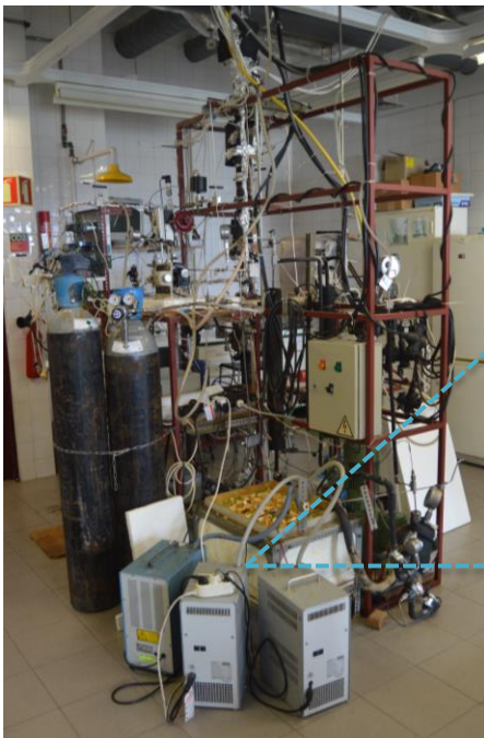
Figure 2.6 – High-pressure installation 1– view from CO 2 bottles and cooling bath.
