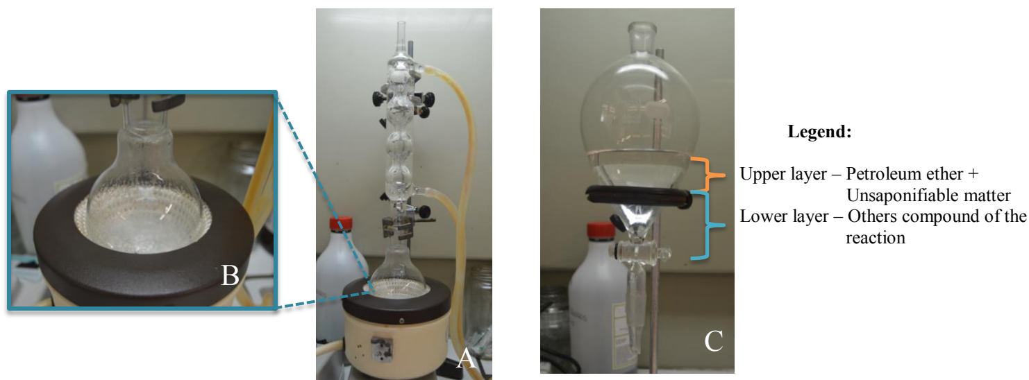
Figure 2.19 – Analysis of unsaponifiable matter. A - Apparatus to proceed the saponification; B - Oil and compounds into the round bottom flask ; C - Separation of the upper layer with a extraction cylinder.
