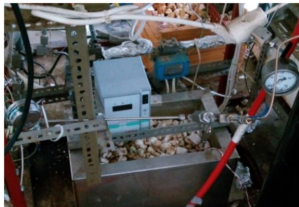
Figure 2.9 – High-pressure Installation 1 - A- Warming bath, B – Static Mixer.
