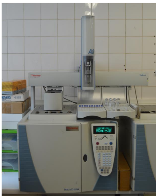
Figure 2.20 – Gas chromatography equipment - THERMO SCIENTIFIC TRACE GC ULTRA.
