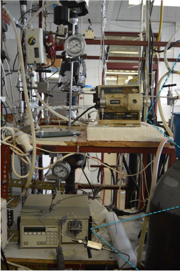
Figure 2.14 – High-pressure installation 1 – view from the oil and methanol pumps (enzymatic transesterification).
