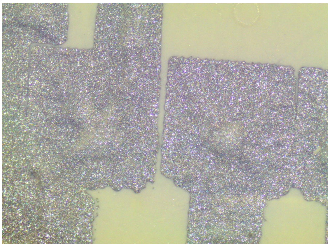
Figure 6.3 – Short circuit on the reservoir area of a 80 \mu\text{m} device
