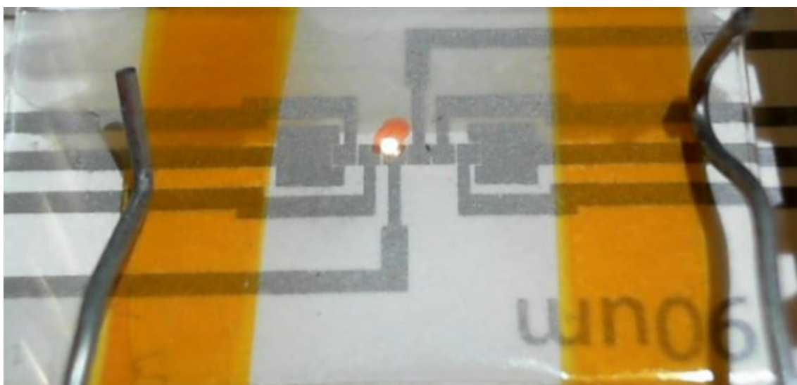
Figure 6.22 – Image of the breakdown during testing of a device with 2 \mu\text{m} Parylene thickness.
