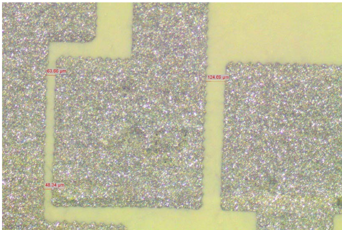
Figure 3.9 – Part of a screen printed circuit, magnified near the reservoir area.
