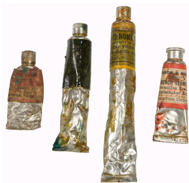
Figure 4. Four of the oil paint tubes analysed by DCR in 2008. From left to right: red carmine (Bourgeois); viridian (Lefranc), chrome yellow (Lefranc) and vermilion (Winsor & Newton) [Melo et al. 2008]
