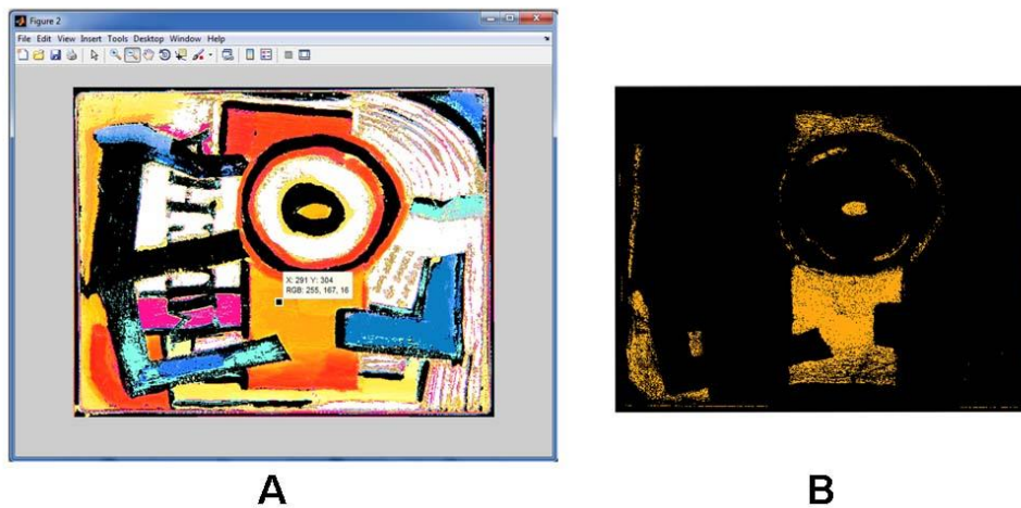
Figure 16. A Selection of a pixel (291; 304) in the segmented image; B mapping of the areas where vermilion and chrome yellow were detected.
