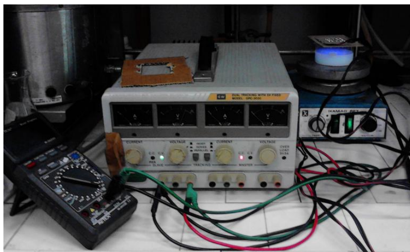
Figure 3.10 Picture of the LEDs experiment (system of volt-ammeter and LEDs connection)
