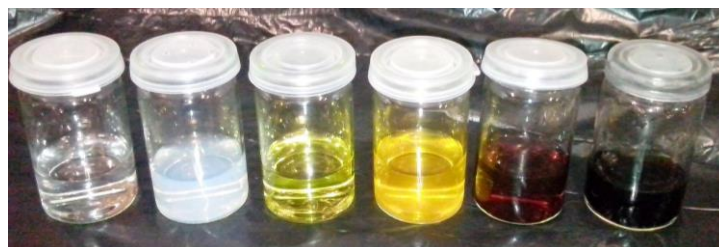
Figure 2.1 – Picture from different solutions prepared for electrodeposition. From left to right: EDOT:PSS, tungsten oxide nanoparticles (WO 3 NPs), commercial gold solution, Au:PVP solution, gold nanoparticles solution, and carbon nanotubes solution.
