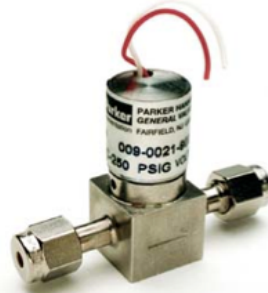
Figure 3-39 - Pressure control valve “Series 9 valve” of Parker®. Maximum operating pressure is 80 bar. The flow coefficient is K_v = 0.005 .
