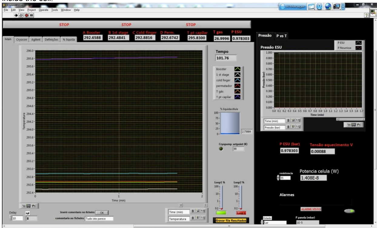
Figure 3-43 - Labview® interface to monitor the pressures and temperatures and control the heaters.
