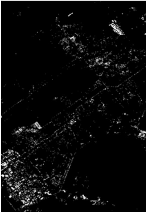
c. Changes between 2003 and 2014 in 6th of October City in binary map using NDVI difference approach
