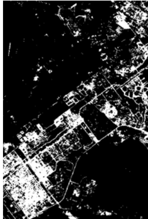
d. Changes between 2003 and 2014 in 6th of October City in binary map using NDVI, NIR and Red differences approach
