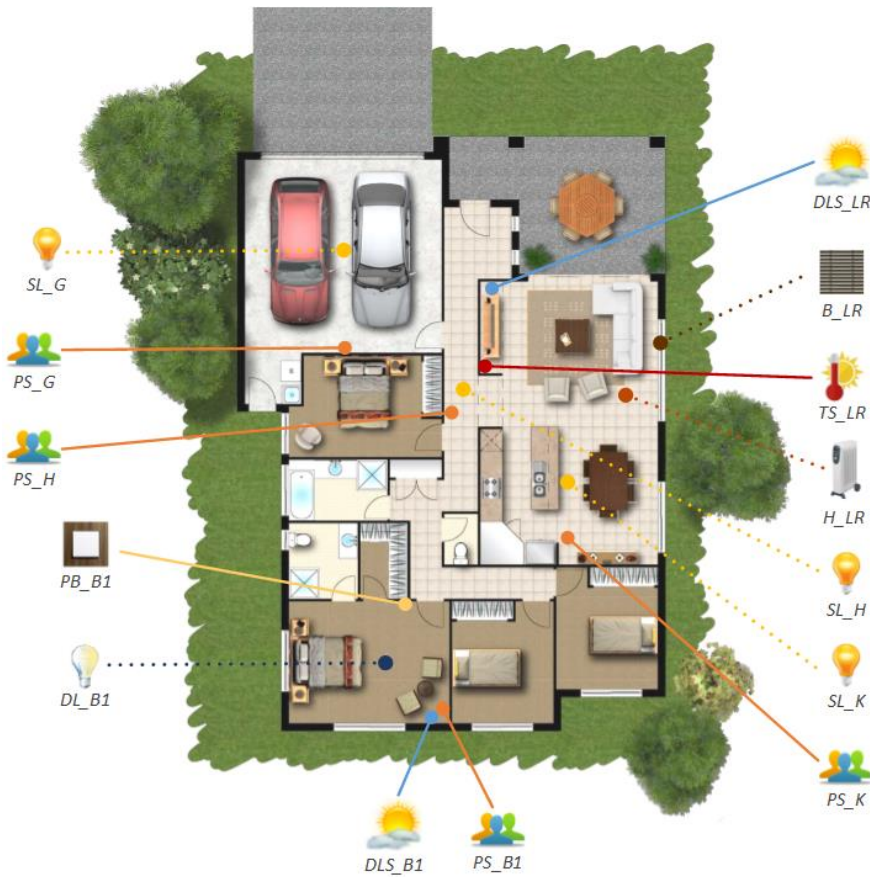
Figure 36 – A floor plan of a habitation with its Sensors and Actuators
