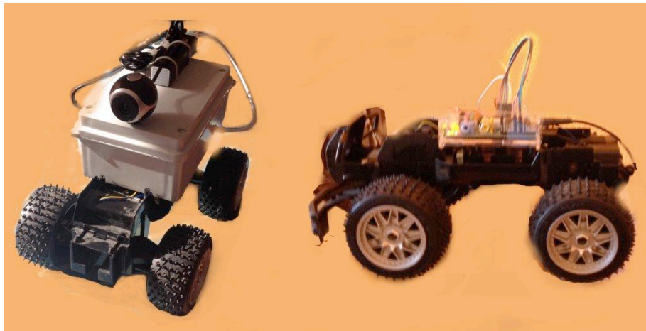
Figure 5.11. PiBot, an adapted remote controlled car to simulate ServRobot.
