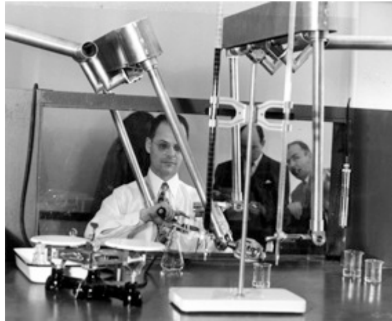
Figure 2.1 Goertz using the first teleoperated system to handle dangerous materials.
