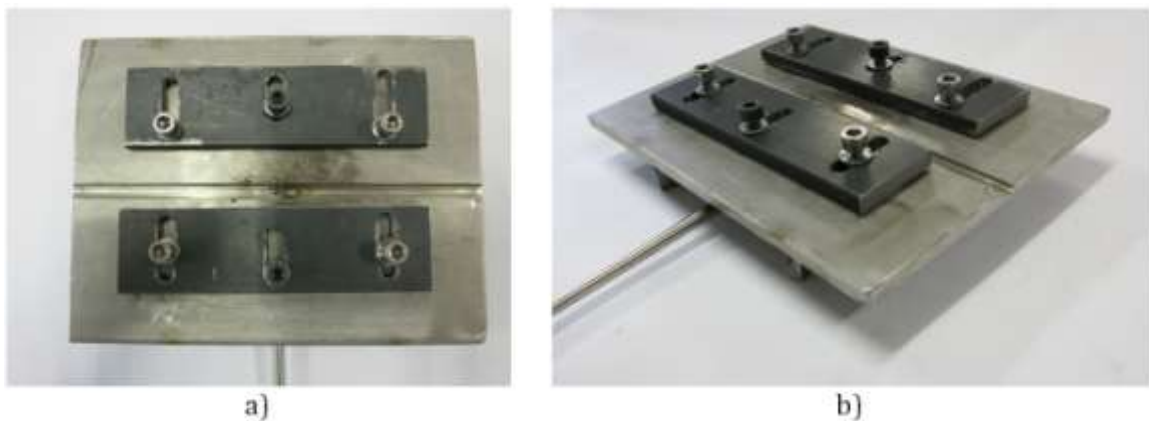
Figure 3.1- a) Top view of the base - central canal and position rulers mounted; b) perspective view of base with position rulers mounted.
