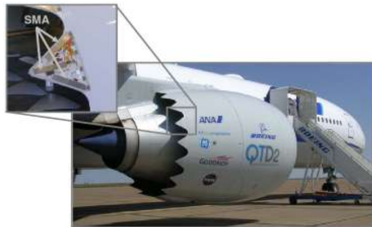
Figure 2.15 - Variable geometry chevron [8].
